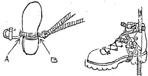
3. Now add the ascender and the brake bar as shown. Be sure the brake bar opens away from the boot.
